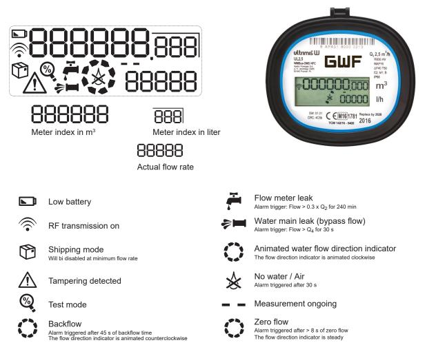
Events not indicated on the LCD: Temperature alarm: If temperature <2°C or >50°C
